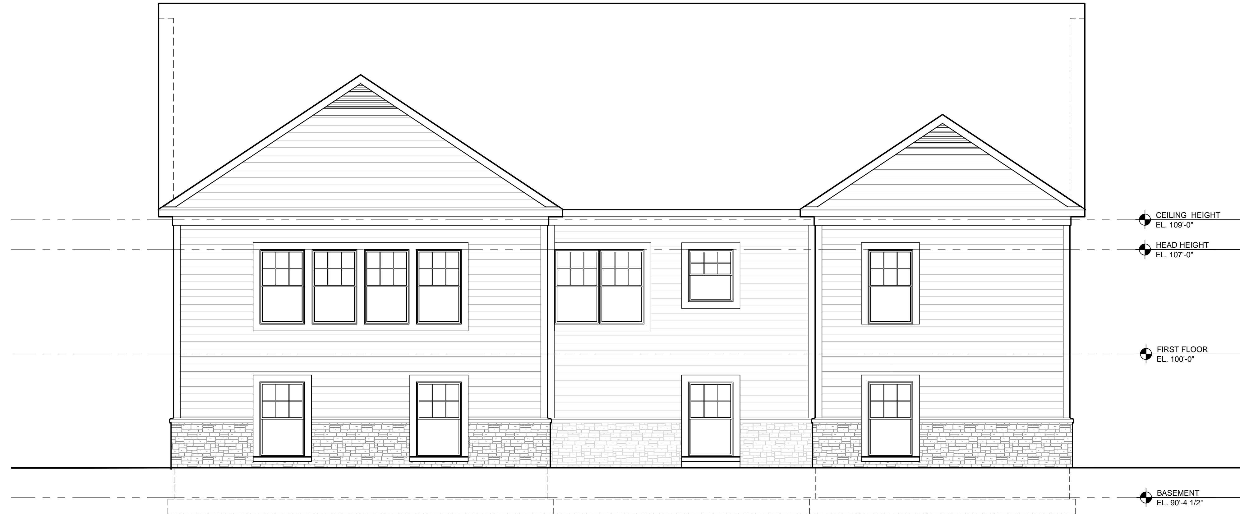
2 Rear Elevation - Michigan - Daylight A2.2 SCALE: 1/4" = 1'-0"
